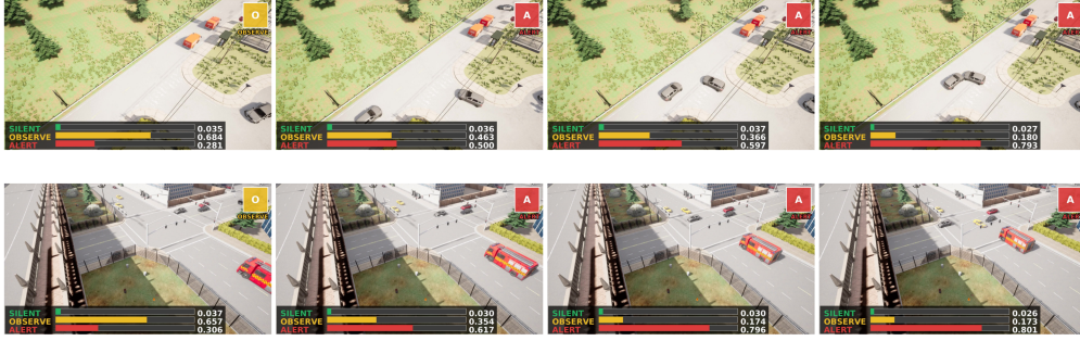
Figure 6: Roadside CARLA accident example. A fixed roadside camera captures an unprotected left-turn collision. VLALERT escalates from OBSERVE to ALERT before impact and sustains the alert, while Gemini remains in SILENT.
